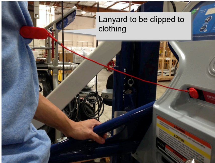
Figure 10. Safety lanyard and magnet location
