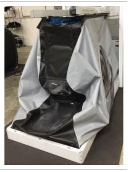
Locate the bag-retaining bars on the frame. The bars on the sides and rear are shown. You will remove these three bars. It may be easiest to start with the rear bar.
