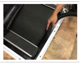
You can also check the surface of the treadbelt for debris or liquid spills. The treadbelt moves freely as you roll it by hand.
