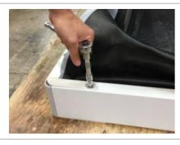
5. The side bars have a slot on the front end, and the slot fits under the adjacent bar. Loosen the fastener on the adjacent bar, and then lift the side bar out.
