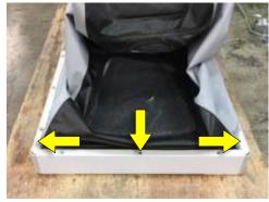
4. Using a socket wrench with a 10mm socket, unscrew the fasteners from the standoffs.
