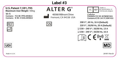
Lifeward, CA Inc.manufactures the system. This label is located on the front panel near the base of the Anti-Gravity Treadmill and identifies the serial and model number of the system, as well as the power and voltage requirements.
