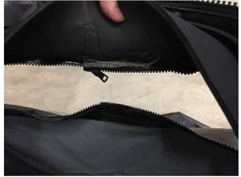
6. Insert the end of the bag zipper into the pull tab on the conning tower zipper, making sure it is fully inserted and the teeth on both zipper halves line up.
