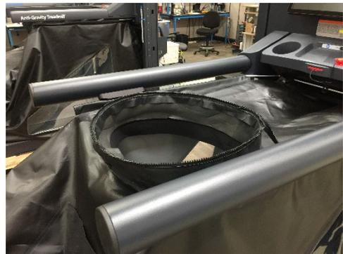
3. Roll back the inside of the conning tower and locate the zipper attachment.
