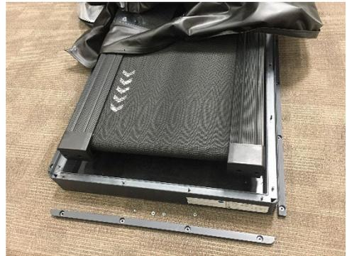
8. You can also check the surface of the treadbelt for debris or liquid spills. The treadbelt moves freely as you roll it by hand.
