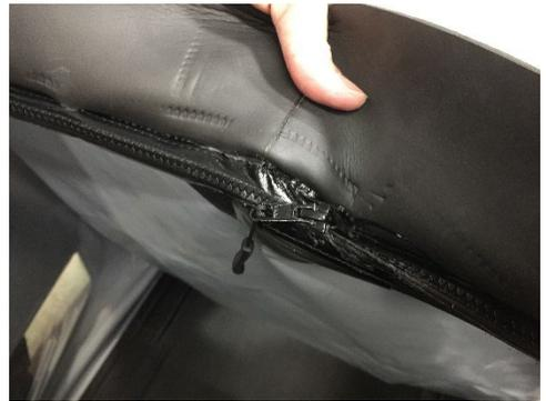
8. Tape the inside of the zipper attachment with 109163 3"x3" tear aid patch or 107588 1-1/2" tear aid strip (3"-4 " length) to seal. Make sure the gap is completely covered.
