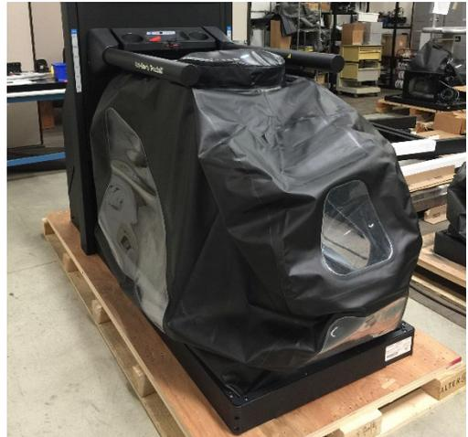
3. Locate the bag-retaining bars on the frame. The bars on the sides and rear are shown. You will remove these three bars. It may be easiest to start with the rear bar.
