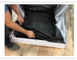
2. Replace the bag-retaining bars on the frame. The side bars must be placed slot-first under the adjacent front bar. Tighten the front bar fastener.
