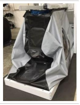
Locate the bag-retaining bars on the frame. The bars on the sides and rear are shown. You will remove these three bars. It may be easiest to start with the rear bar.
