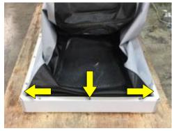
4. Using a socket wrench with a 10mm socket, unscrew the fasteners from the standoffs.
