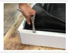
5. The side bars have a slot on the front end, and the slot fits under the adjacent bar. Loosen the fastener on the adjacent bar, and then lift the side bar out.
