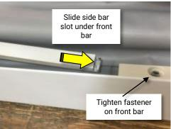
3. Replace and tighten all fasteners. Make sure they are snug. **Do not over-tighten**.
