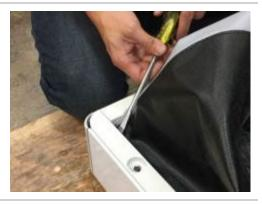
7. Pull the bars completely off the frame and set aside with the fasteners.
