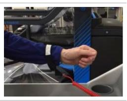
2. Place the lanyard safety magnet directly over the circular indicator on the console labeled "Emergency Stop"; otherwise, the Anti-Gravity Treadmill will not operate.
