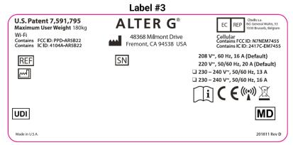
AlterG manufactures the system. This label is located on the front panel near the base of the Anti-Gravity Treadmill and identifies the serial and model number of the system, as well as the power and voltage requirements.
