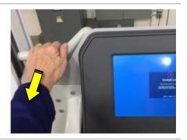
Grasp the handrails and slide the cockpit up or down to set it at a height that places the zipper at the iliac crest (the top, outer edge of the pelvic bone felt just below waist level). For additional trunk support, the cockpit can be set higher.
