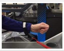
2. Place the lanyard safety magnet directly over the circular indicator on the console labeled "Emergency Stop"; otherwise, the Anti-Gravity Treadmill will not operate.
