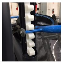
8. Close the safety latches located on the 2 front height adjusters. Press the latches down all the way and secure them with the spring-loaded safety pins.
