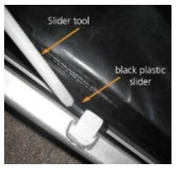
4. After you slide out all the plastic tabs on the frame, tilt the metal slat towards the inside of the treadmill. In the locked down position, the metal slat should be at a 45degree angle pointing towards the outside of the treadmill. You may have to push down on the slat as you rotate it inwards.
