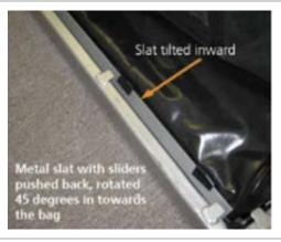
5. Lift the slats and pull them out. Collect the black plastic tabs. There are 28 tabs: 10 on each side, 4 on the front, and 4 on the back.
